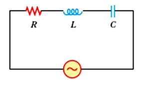
small,  $X_C = \frac{1}{\omega C}$  is much greater than  $X_L = \omega L$ . So the capacitance dominates at low frequencies and circuit behaves like an RC circuit.
