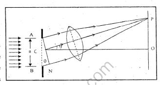
To find the value of path difference, draw a normal "CO" on the screen from the mid point "C" of the slit. If the diffracted light is focused at "O", brightness will be obtained because the rays reaching at "O", from all points of the slit will cover equal path.
