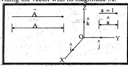
Unit vectors along x, y and z-axis are denoted by i, j and k respectively.
