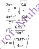
This is the expression of a geostationary orbit of a satellite.
