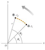
Let  $\Delta \theta$  is the angular displacement during the time interval  $\Delta t$ , the average angular velocity during this interval is:
