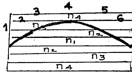
fig (g) Light propagation within a hypothetical multi layer fibre.
