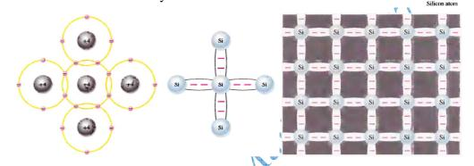
The semiconducting materials have negative temperature coefficient of resistivity. At low temperatures, the valence band is completely filled and conduction band is completely empty. Thus the semiconducting materials behave like insulator at low temperatures.
