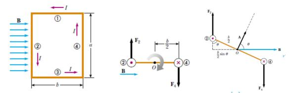
We want to find out the expression of torque produced in current carrying coil due to the effect of magnetic field.
