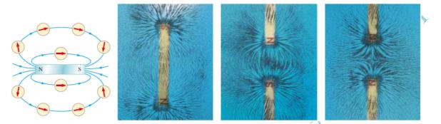
In addition to a bar magnet, a moving charge or a current creates a magnetic field in the surrounding space (in addition to its electric field). The magnetic field exerts a force F on any other moving charge or current that is present in the field.
