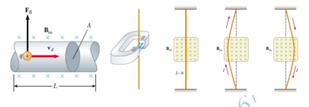
If n is the number of free charges per unit volume of a conductor (each having charge e), then the total charge flowing through the wire is q = nAle.
