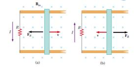
If the bar is moving to the left, as in figure (b), the external magnetic flux through the area enclosed by the loop decreases with time. Because the field is directed into the page, the direction of the induced current must be clockwise.
