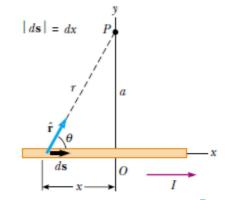
is at the distance x from point O (taken as the origin). The magnetic field strength due to length element ds by Biot-Savart law will be:
