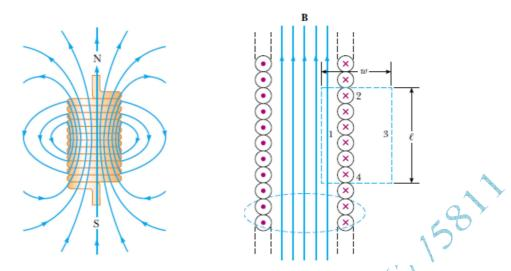
We want to find out magnetic field intensity  $\mathbf{B}$  at point P inside a current carrying solenoid. For this we consider an Amperian loop. The symmetry shows that the close path can be divided into four elements 1, 2, 3 and 4. By Ampere's law:
