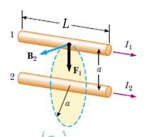
The wire 2, which carries a current  $I_2$  creates a magnetic field  $B_2$  at the location of wire 1, which can be find out by using the expression:
