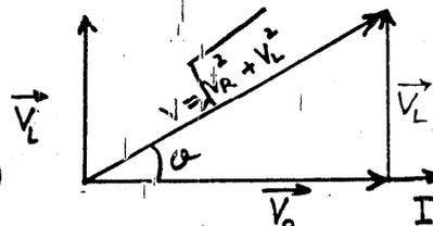
Q.16.7 A choke coil placed in series with an electric lamp in an A.C. circuit causes the lamp to become dim. Why is it so? A variable capacitor added in series in this circuit may be adjusted until the lamp glows with normal brilliance. Explain, how this is possible?
