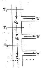
The 2nd engine recieves heat Q2 at temp. T2 and rejects heat Q3 to the third engine and so on.
