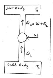
In a perfect refrigerator N=0 and so  $Q_1=Q_n$ . So the coefficient of performance of perfect refrigerator is infinity.
