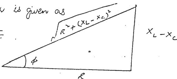
According to eq. (1) average power dissipated is maximum when  $\cos\phi$  is maximum. But  $(\cos\phi)_{max} = 1$ .
