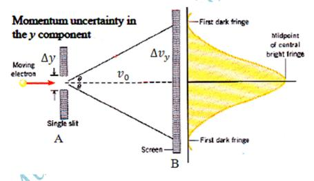
Due to the wave nature, the electron beam bends on the either side of the central point producing the diffraction pattern. Let  $\Delta v_y$  is the uncertainty in the component of velocity along y axis for the first minimum, then we have
