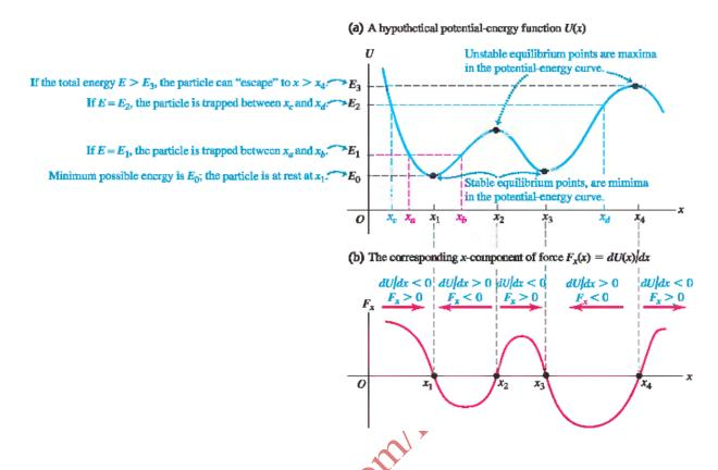
The slope of the U(x) curve is also zero at points  $x_2$  and  $x_4$ , and these are also equilibrium points. But when the particle is displaced a little to the right of either point, the slope of the U(x) curve becomes negative, corresponding to a positive  $F_x$  that tends
